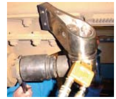
Patented Multi-Axis Swivel provides better accessibility and prevents hose kinking.
